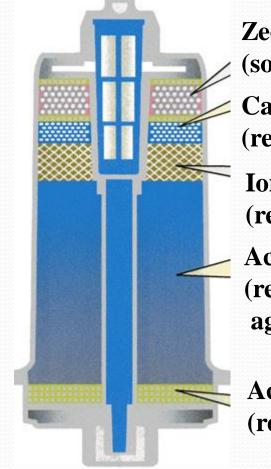
Zeolite Ball Ceramics (soften water) Calcium sulfite (removal of free chlorine) Ion exchange resin (removal of lead) Active carbon with silver (removal of odor, trihalomethanes, agriculture chemicals, etc.)
